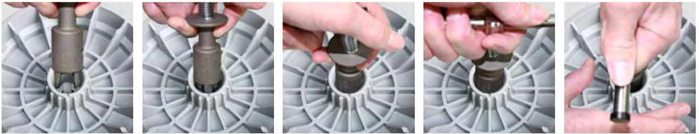
Figure 11: Place Filtrate Isolation Valve Tool over valve stem in Top Cap. When attached to valve stem, valve can be rotated clockwise to unlock it.
