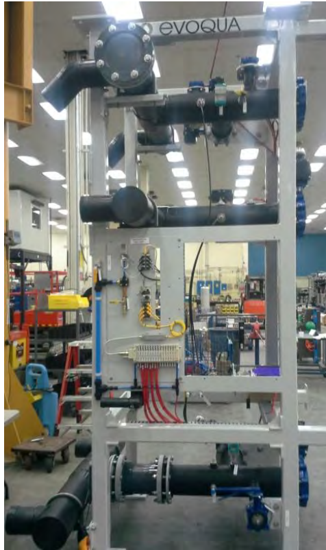
Figure 2. Piping Skid Assembly in Colorado Springs, CO
