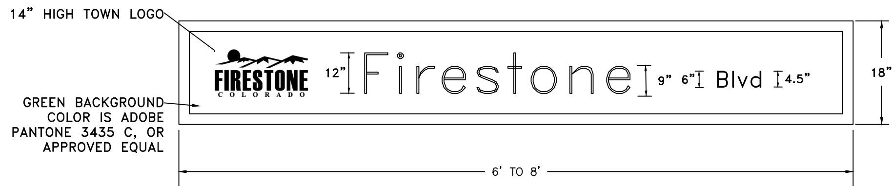
LIGHTED SIGN TYPICAL LAYOUT
