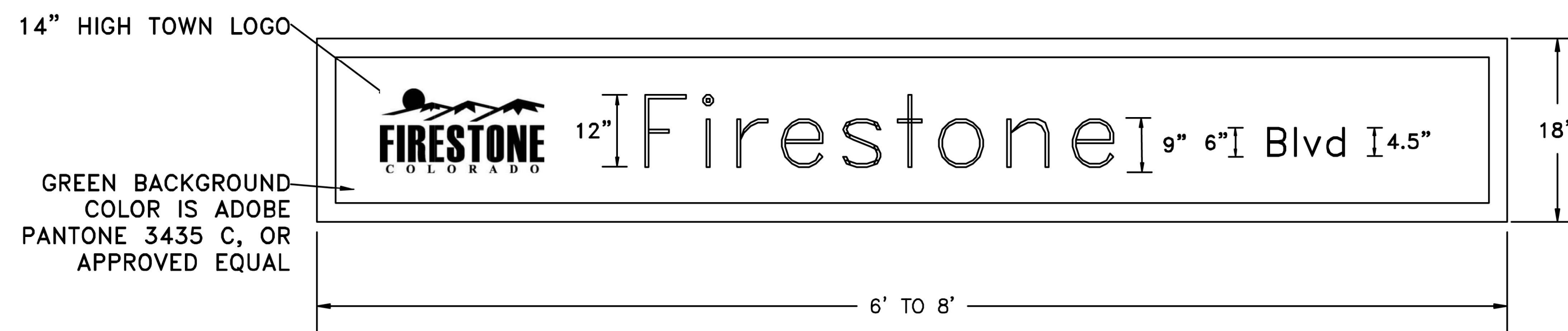
LIGHTED SIGN TYPICAL LAYOUT
