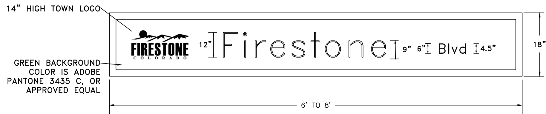
LIGHTED SIGN TYPICAL LAYOUT
